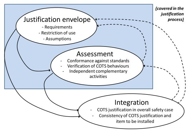
Figure 1. Typical flowchart for a COTS justification
