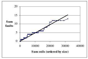
Fig. 5. Logic faults vs. network coils (cumulative)
