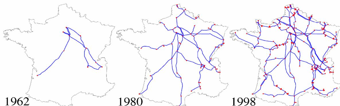
Figure 5: Topology of the French high voltage electricity network for selected years
